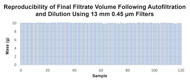
Measured mass of 120 10X diluted filtrates, automated using **TRAX**Station. 1 mL of sample was drawn into the LuerProbe then diluted with 9 mL of 2% HNO<sub>3</sub> through a 13 mm 0.45  $\mu$ m Luer filter. The target mass of the prepared sample in the tube was 10.07 g. The average measured mass was 10.06 g with an RSD of 0.75%, indicating the high reproducibility of the high throughput approach to filtration and dilution.
